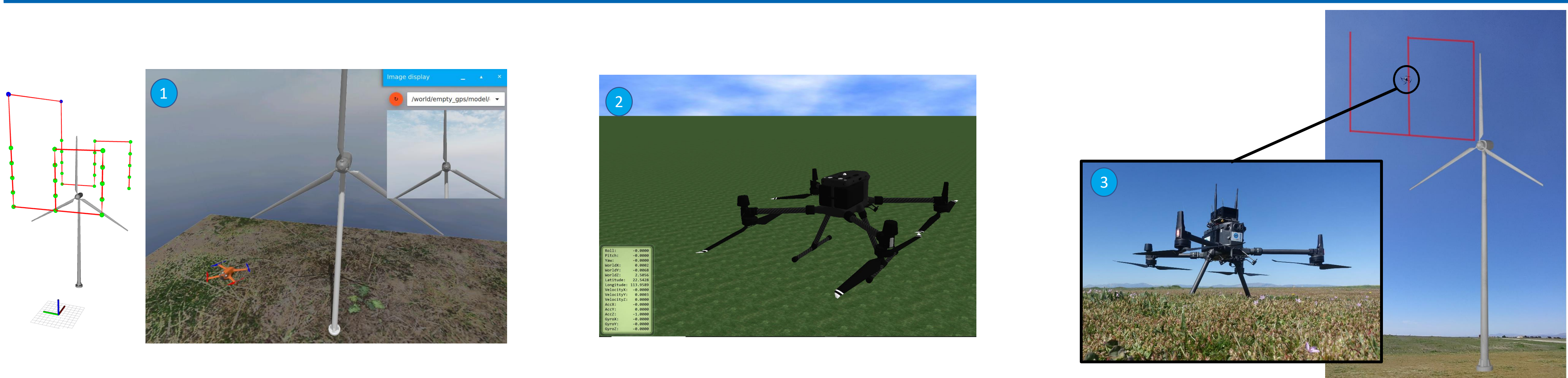
Gazebo Simulator for Wind Turbine inspection and RViz visualization of the inspection trajectory waypoints
