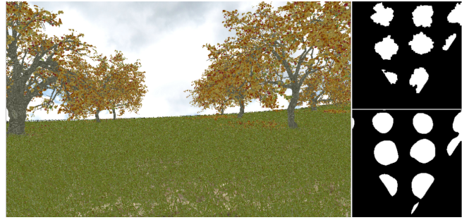
Fig. 5: Prediction/Test of the PYVA method on an apple orchard in autumn . The network was trained with 1200 images of an apple orchard in summer.
