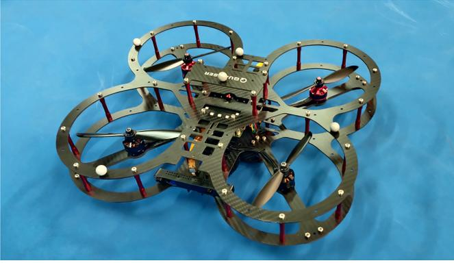
Fig. 1: QDrone research UAV from Quanser. The dimensions of the QDrone are  $40 \times 40 \times 15$  cm, the mass is 1.21 kg, and a motion capture system connected over WiFi is used for position measurements.
