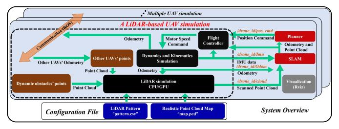
Fig. 2. The overall framework of our simulator (black dashed box) and how it interacts with external modules in ROS.
