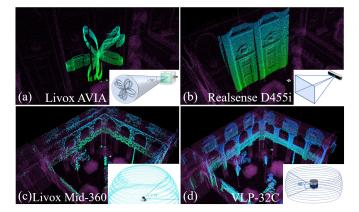
Fig. 5. Various LiDAR scan pattern support including Livox Avia (a), D455 (b), Livox Mid-360 (c), and VLP 32 (d), respectively.
