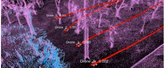
Fig. 7. Multi-UAV planning simulation. The pink models are the UAVs, and the red curves are the trajectories of the UAVs, avoiding the obstacles of a realistic forest map.
