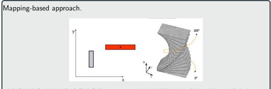
Left: Robot (red) and obstacle (grey). Right: Configuration space; each polygon is Minkowski sum of robot and obstacle at fixed orientation.
