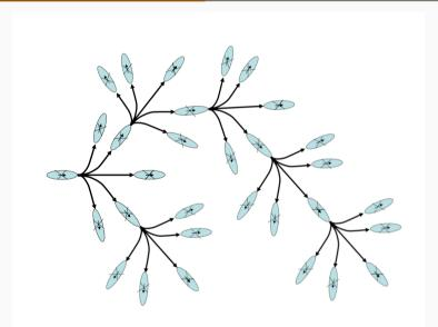
Idea: Define nodes as transitions from previous nodes. Use precomputed motion primitives to expand a node.
